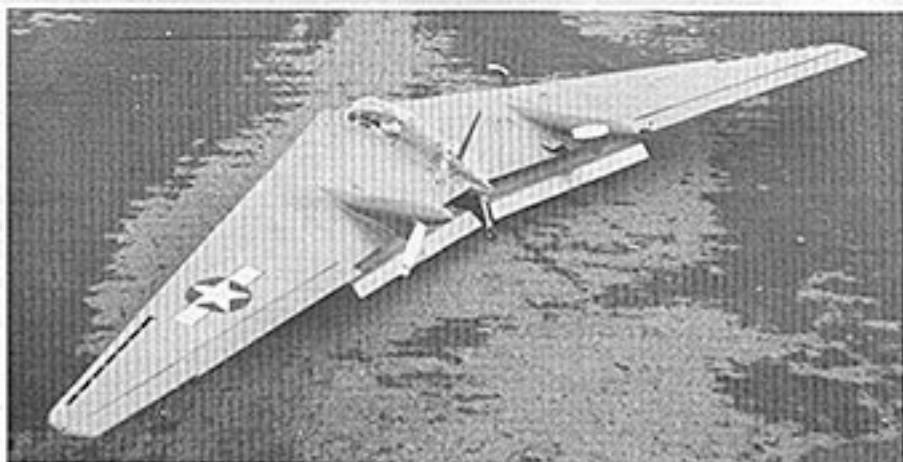
N9M-A model on static display with landing flaps deflected. Top of the aircraft is a medium blue, the bottom is orange-yellow. Model does not feature the split surface yaw control.
