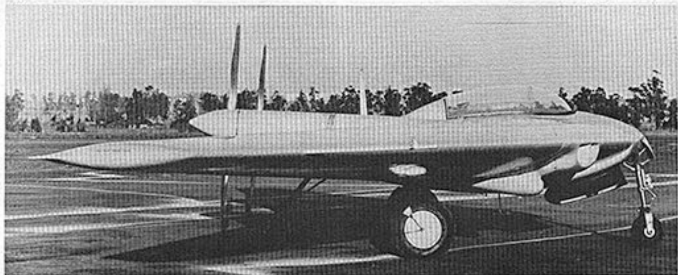
Right side view of N9M-2 at Northrop Field, Hawthorne, California. Slats were added to leading edge later in flight testing to cure slow speed/high attack angle tip stall. N9M-A and -B featured built-in slats.
