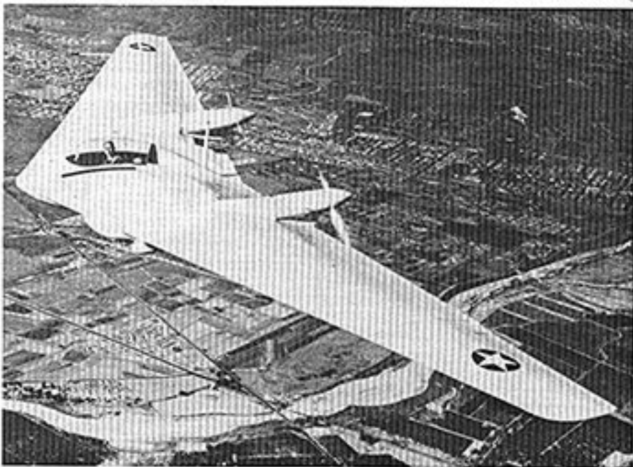
Wouldn't you love to have seen the N9M-2 flying wing up this close on one of its flight tests over Southern California? Note lack of L.E. slots or slats to prevent tip stall.
