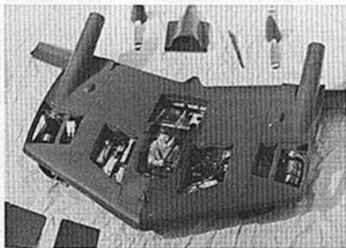
Five hatches cover all of the model N9M-A's innards. Let's see . . . 05 motors, fuses, retracts, motor control switch, nose gear servo . . .
