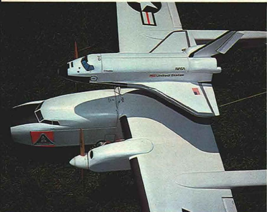
The tall wire launch frame was meant to ensure that the Shuttle would clear the tail of the carrier plane. It didn't turn out to be a problem; a shorter frame would also work well.
