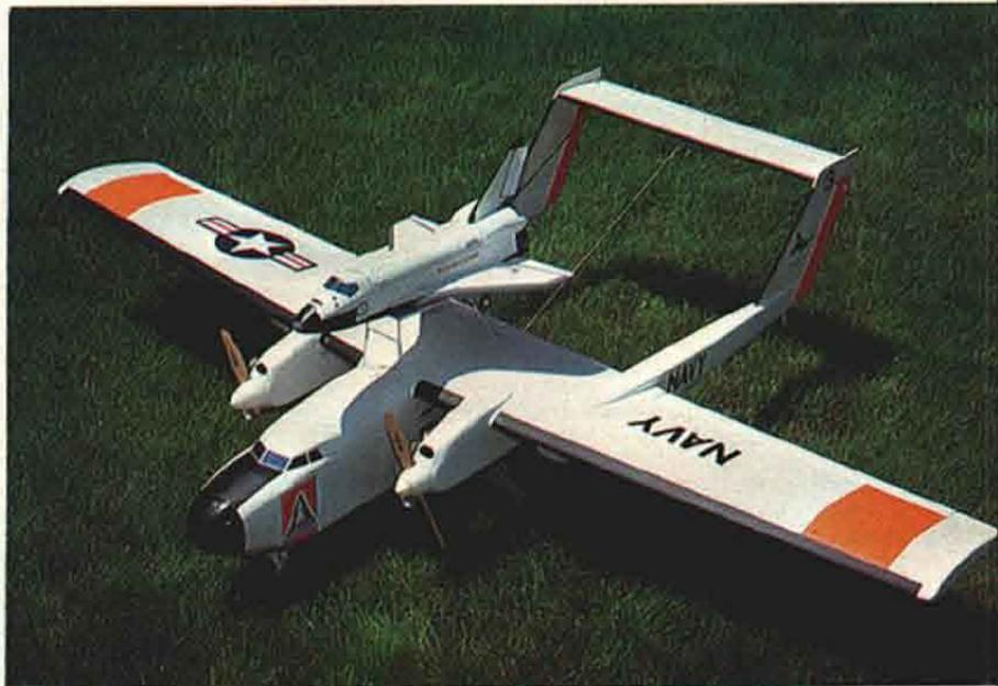
The paint schemes of these two unique flying machines almost match—look at the noses! High stab on the Twin is to allow a drag chute to be released out of a hatch on the fuselage.
