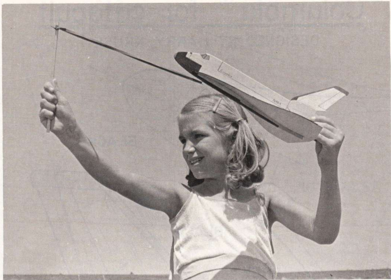
Kerri Kruse, 8, shows the proper launch position for the shuttle craft. The dowel handle is 1/4 inch stock; the launch rubber is 3/16 or 1/4 inch.
