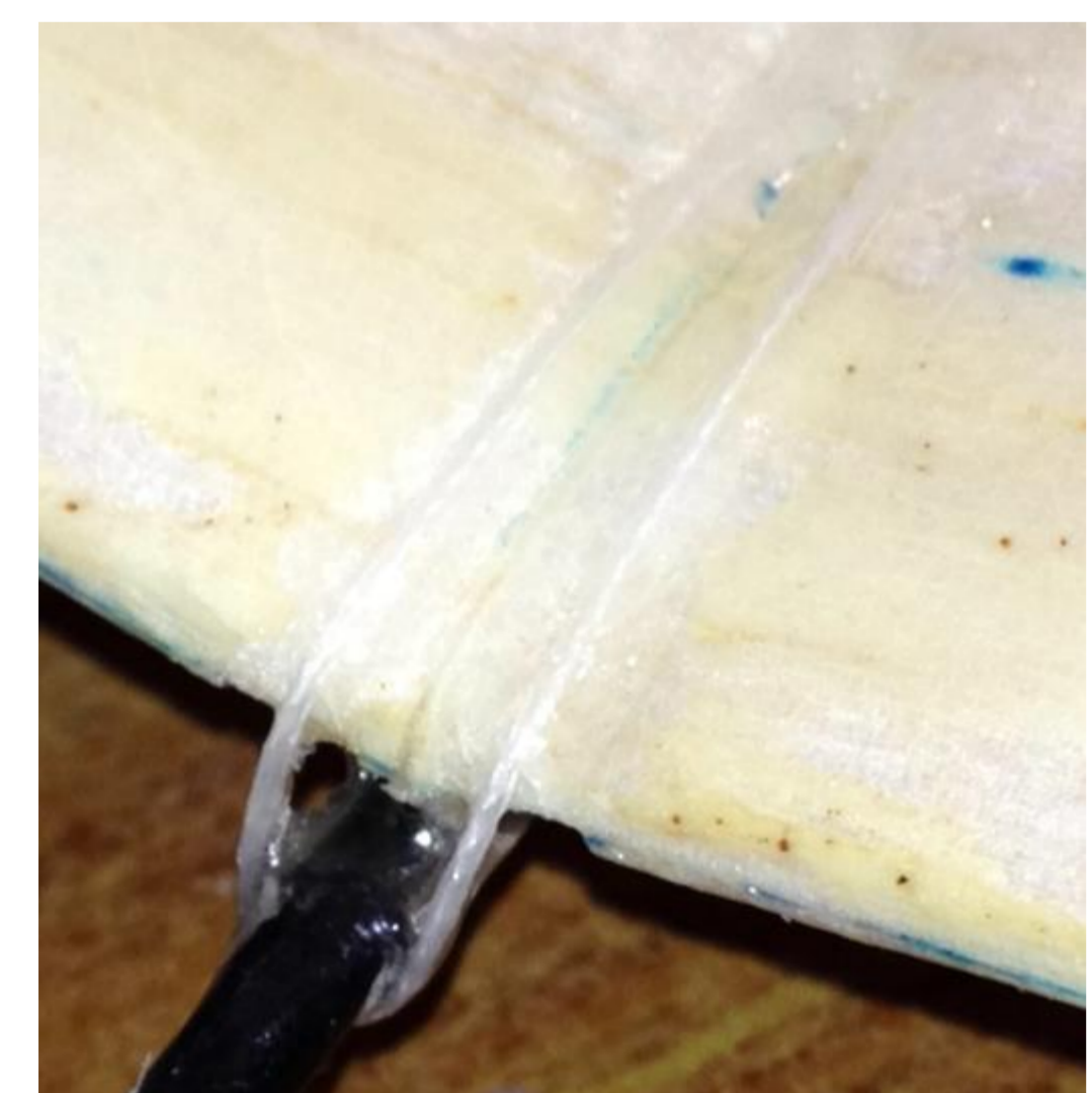
Glue wing and body with 2 drops of cyanoacrylate instant adhesive. Glue backing line of fly fishing with epoxy adhesive. Reinforce with epoxy adhesive around them.
