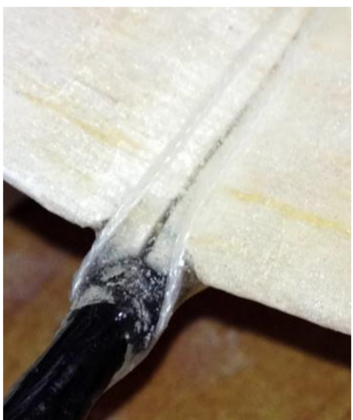
Glue wing and body with 2 drops of cyanoacrylate instant adhesive. Glue backing line of fly fishing with epoxy adhesive. Reinforce with epoxy adhesive around them.
