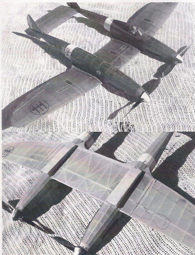
Fig. 9 Underside of model showing three-piece wing. Bill uses same propellers as in Arado 530, see FFQ#18.
