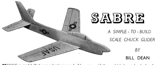
HERE'S a model that even a beginner can build in a couple of hours—a profile of the famous Sabre jet fighter. We chose the F-86D version because of its long radar nose and easier-to-make flat tailplane. All patterns are shown full size, so just trace or pinprick them on to medium weight  $\frac{1}{16}$  in. and  $\frac{1}{8}$  in. balsa sheet. Cut out with a sharp razor blade and make two wing panels.
