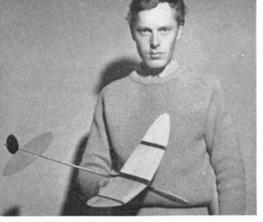
1 loop and right-spiral climb under power, tending to nose up if the turn over-tightens and (2) a very flat, safe left glide circle.
