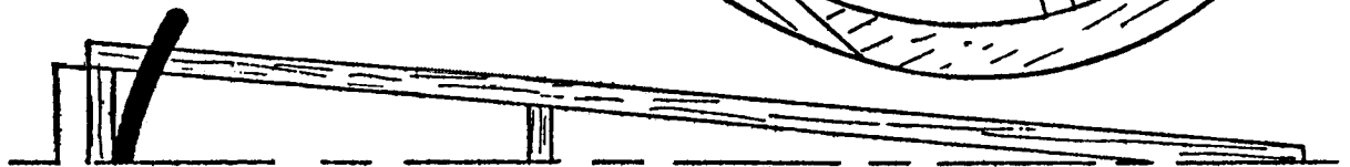
tail piece held to fuselage by rubber bands
