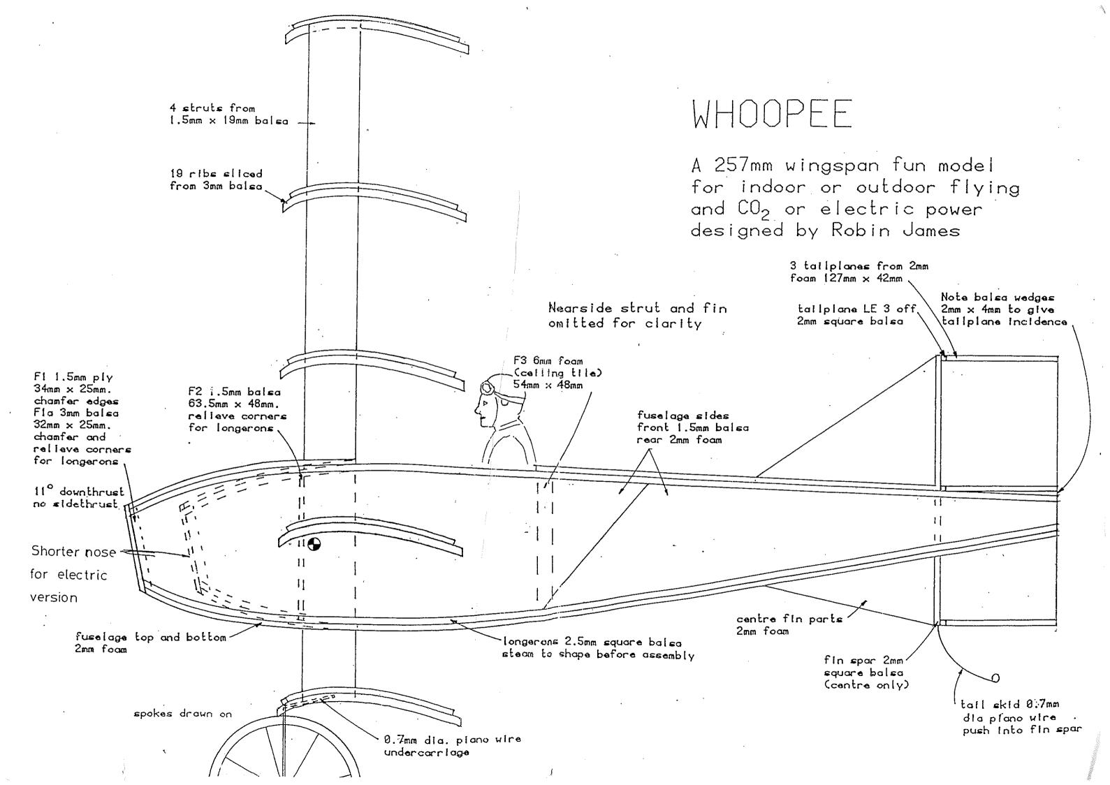
cut 5 wings from 2mm foam, 254mm x 64mm note slots for centre struts:
