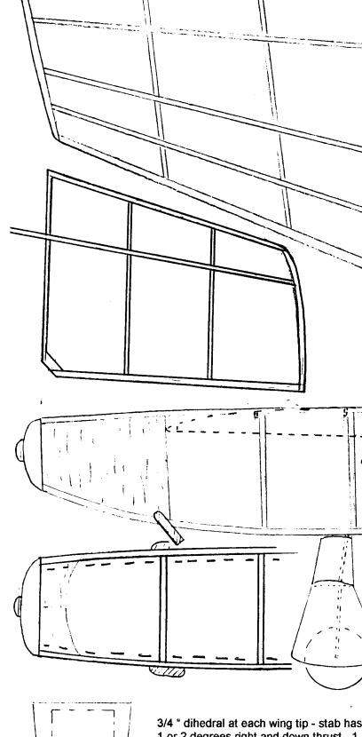
3/4 " dihedral at each wing tip - stab has 1 or 2 degrees right and down thrust. 1 in left wing. Wing tips have sanded in w is tapered from bottom). A 6" Hi Flier so is a 25" loop of 1/8 or 5/32 rubber.
