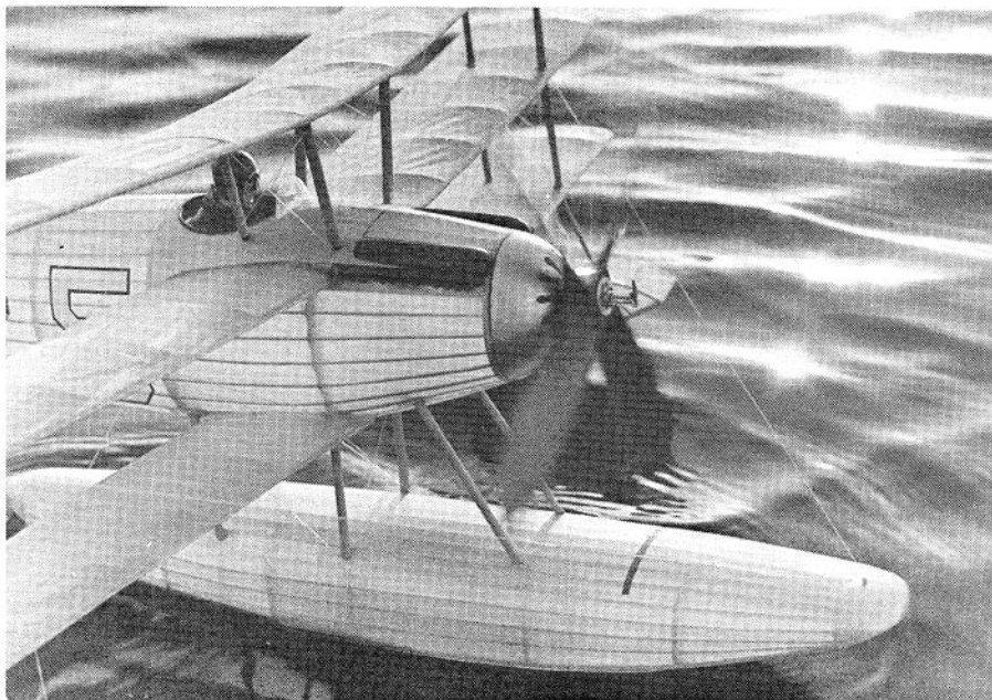
Bill used a freewheeling device on the prop for longer flights. Some of the struts are made from cocktail straws. Monofilament "wires" add greatly to the model's strength.
