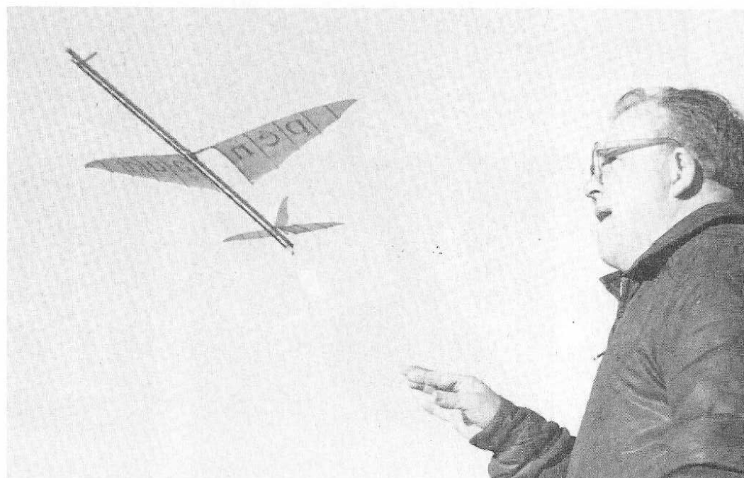
Walt Mooney launching Bill Hannan's planophore. At a Flightmasters West Indoor contest, Walt proxy-flew Bill's planophore for an officially clocked 58-second flight. The model weighs 16 grams, about equal to a Pénaud original. It's built from basswood and is tissue covered.
