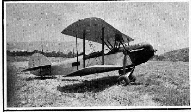
Fabric covered landing struts makes this Waco unusual . . . note radiator mounted below center wing section.
