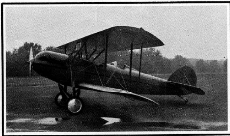
Waco 10 with good view of original wheels, has faired cowling and carries NC number 904H.
