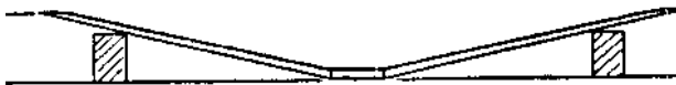
FIG. 4 RAISE WING-TIPS AS SHOWN, TO OBTAIN DIHEDRAL WHEN ASSEMBLING THE TWO HALVES.
