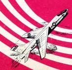
Powered by a Pratt & Whitney J-57-P4 with afterburner, the "Crusader" holds America's speed record of 1,015 mp.h. & has made the fostest transcantipental flight to date. The first corrier aircraft to exceed 1000 m.p.h.
