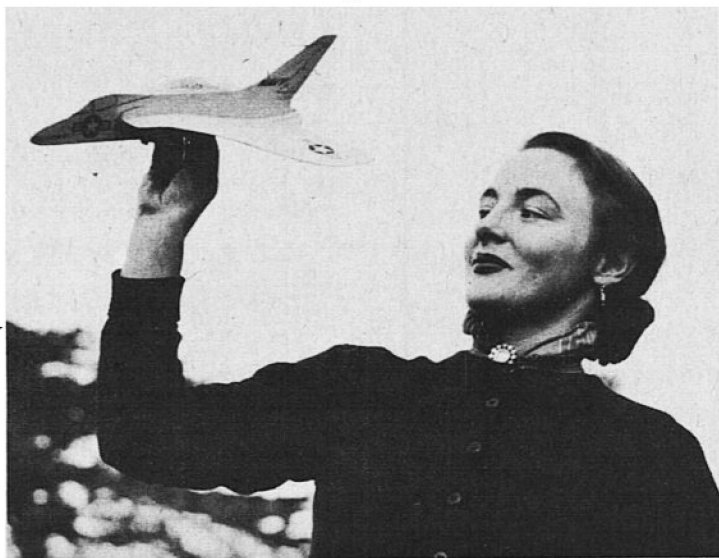
Pretty in flight is the tiny Skyray here held as for launching by Val Mason. Odd fact about deltas is their stability without dihedral. Sweepback has same effect.
