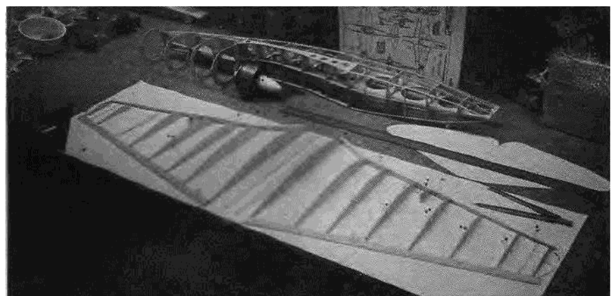
Wing construction before addition of spars.
