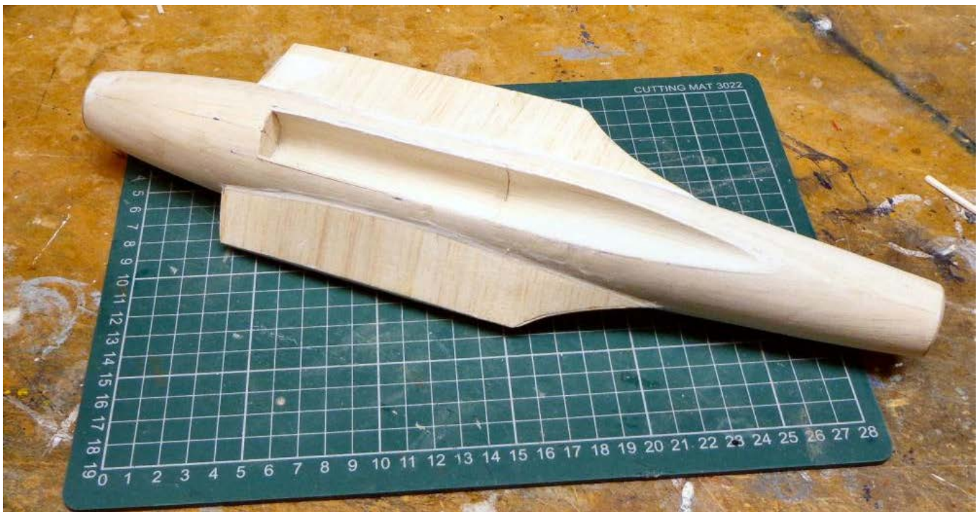
Above: the fuselage (at last!) nearly finished. At this point it weighs 18g and just needs the nose block, tail pipe and smoothing down.
