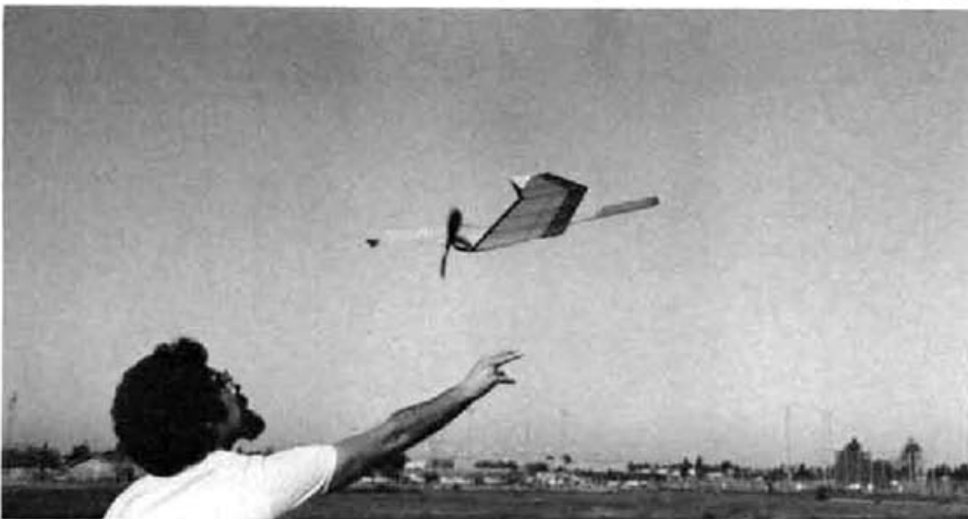
The author launches his Swallow at Mile Square Park in Fountain Valley, California. The model should be launched with wings level in a slightly nose-up attitude.
