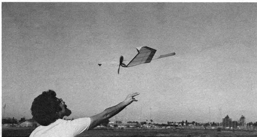
The author launches his Swallow at Mile Square Park in Fountain Valley, California. The model should be launched with wings level in a slightly nose-up attitude.
