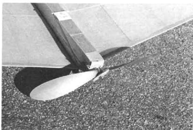
Rear view of Swallow shows plywood prop drive unit required to comply with "unmodified propeller" rule. The drive unit fits over the back of the prop, but is not permanently attached to it.
