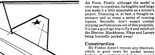
My Foxbat doesn't require any titanium, which is good news for pocket money budgets. Its constructional style owes a lot to the far superior foam aircraft produced by Rick Grainger of Nottingham MAC. In essence, a fairly minimal balsa structure is covered in panels of 2mm polystyrene insulation with all the relevant panel lines inked on prior to assembly. The 2mm foam is available in large rolls from hardware stores. 50p
