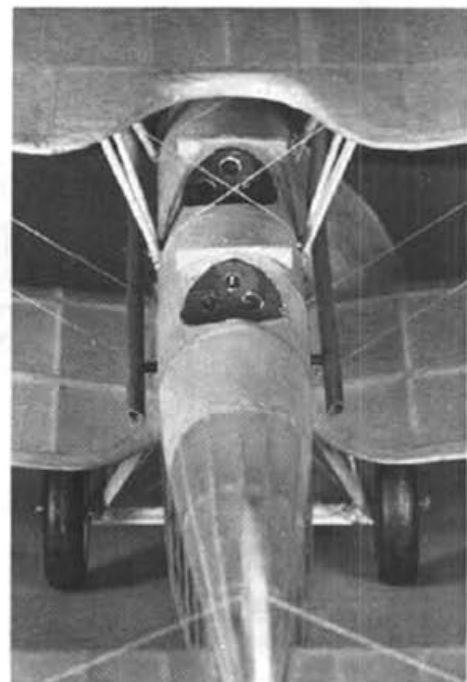
Rudder's eye view of the cockpit. Exhaust pipes bent from aluminum tubing.
