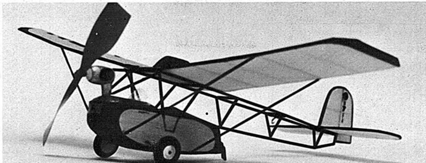
One thing about the 'Tub', it's no trouble replacing the rubber motor! Author uses styrofoam parts to keep weight down.
