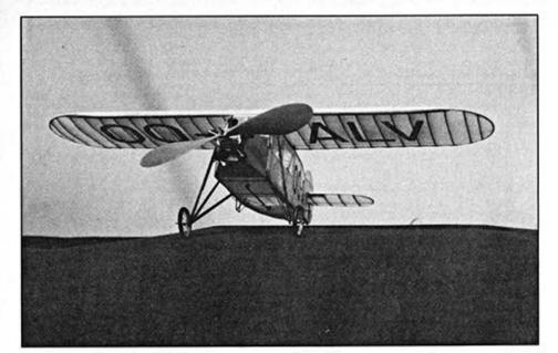
Don't worry about the lack of dihedral, the Renard flies well without it. Walt designed it with scale rib spacing and a very nearly scale structure, but explains how you can safely eliminate some of it to make a lighter and therefore longer flying model.
