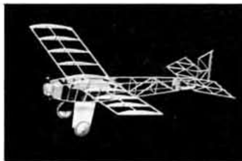
A view of the Farman before covering with tissue. Model is just held together with scotch tape for picture.
