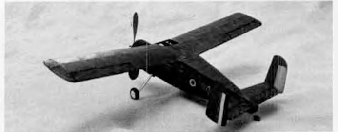
Build this model with lots of downthrust because of the relative small size of the horizontal stabilizer.
