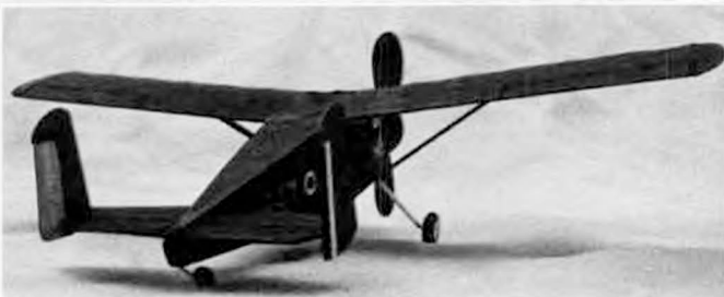
One of the distinguishing features of this model is its twin vertical stabilizer design. Tail wheel pivots for scale-like appearance.
