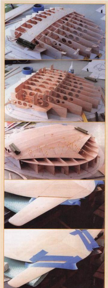
Top planking started. Note the two pieces of bottom planking in place to hold the structure true. There are spacer tabs at the rib ends. Use 1-piece skin planks as much as possible.
