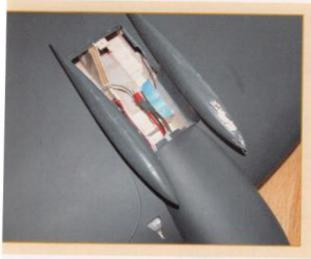
The bottom view shows the access hatch between the permanently-mounted drop tank skids. Batteries end up under aft edge of hatch to give proper balance.
