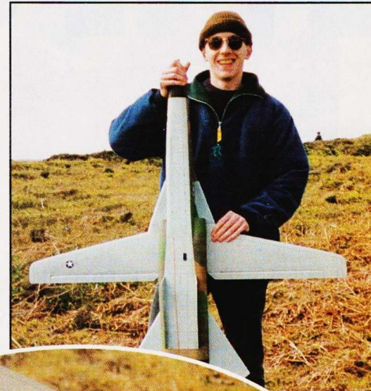
RIGHT: Phil finished the model the night before the competition! Here he proudly displays the lower surfaces -note the ventral strakes, cheek intakes and the coffee cup tail pipes!
