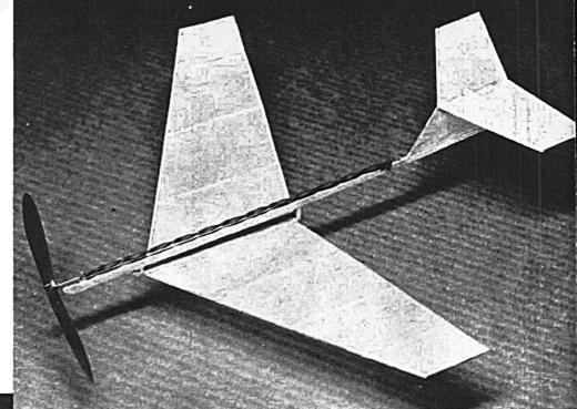
Paper is not sprayed or dope coated on such small models. Builder used nail polish to attach paper edges—because of the small brushes!
