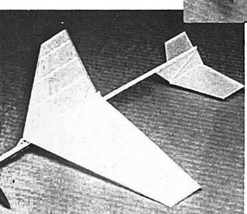
Inverted view. Cover model in temperature approximately same as that where it will be flown—paper pulls when warmed, loosens when cooled.
