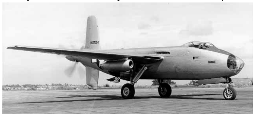
The DC-8 Skybus was patterned after the Douglas XB-42A. Note the double bubble, "bug-eyed," canopy design. (Douglas photo from The Boeing Company)
