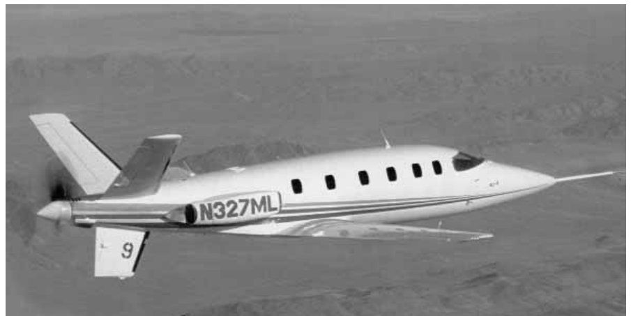
Similarly unsuccessful to the Skybus, the Lear Fan differed in that it used two engines to drive a single pusher propeller. (1983 Lear Avia photo from the Earl See collection)
