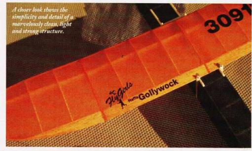
endeavour for you. Longerons are stiff and springy 7-pound 1/16" strip and the uprights and spreaders do well as 4/5-pound stock. I use 5-pound "C" grain 1/32" sheet for all ribs, fillers, rudder and gussets. The nose block is cross-laminated from 5/7-pound 1/16" sheet.
