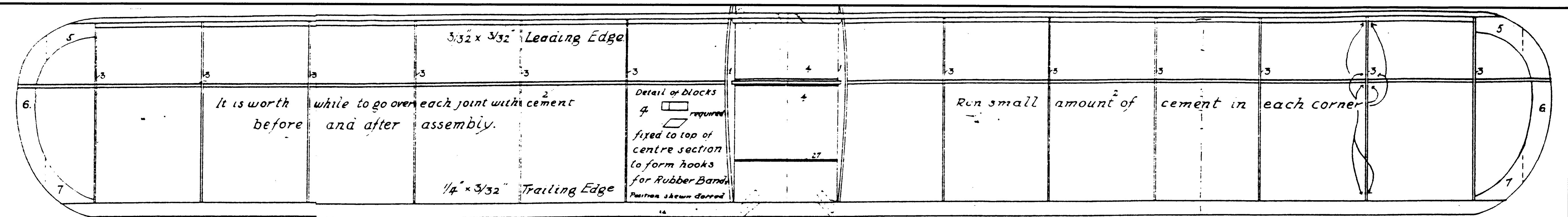
Before joining together the 2 halves of MAINPLANE, you must cut away the underside of the trailing edge on the correct bevel so that the centre ribs No.1 sit flat along their length, when the wing tips are raised  $2\frac{3}{4}$ . SEE X.X.
